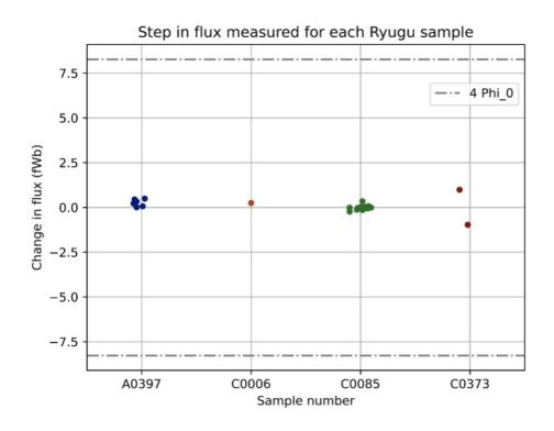
Summarized results of 24 pass-through experiments conducted on returned Ryugu samples A0397, C0006, C0085, and C0373. Here,  $\Delta\Phi$  is expressed in terms of fWb. The dotted-dashed line represents  $\Delta\Phi$ 0 = 8.23 fWb, which is the minimum quantized charge in flux expected by a Dirac magnetic monopole. Since  $\Delta\Phi$ 0 of all samples is much lower than 4 $\Phi$ 0, we have not yet detected a magnetic monopole.
