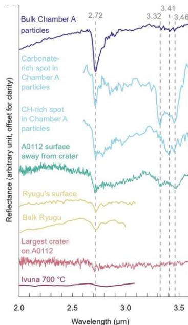
Figure 2. Reflectance spectra obtained from inside the largest impact crater on A0112 (red) compared against a spot far away from the craters (green). Also shown are spectra of bulk A particles (dark blue [13]), carbonate- and CH-rich spots on Chamber A particles (light blue [13]), Ryugu's bulk surface (yellow [15,16]) and heated Ivuna CI chondrite (pink and red [14]) for comparison.
