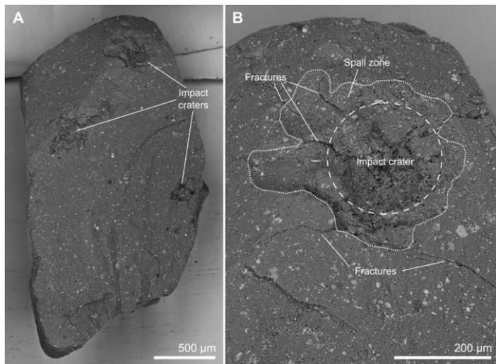
Figure 1. SEM-BSE images of the crater-covered side of A0112 (A) and the largest impact crater surrounded by a spall zone and surface-related, impact-produced fractures (B).
