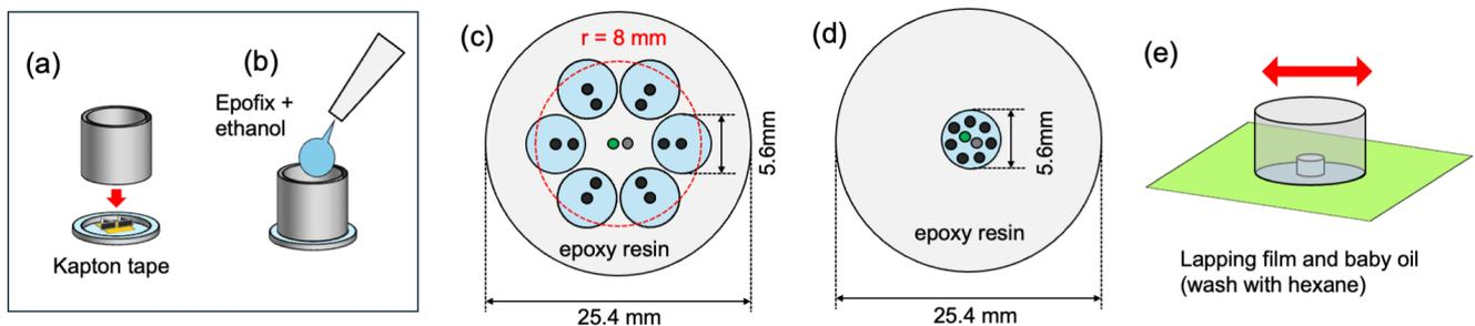
Figure 1. Production of SIMS mounts. (a) placing the fragments on Kapton tape, (b) add the mixture of Epofix and ethanol and cure. (c-d) Schematic view of sections with multiple unknown samples (7-13) and SIMS standard at the center. All samples should be within 8 mm from the center of the mount for high precision stable isotope analyses [4]. (e) The surface of the samples was polished using lapping film with mineral oil as the lubricant, followed by hexane wash.
