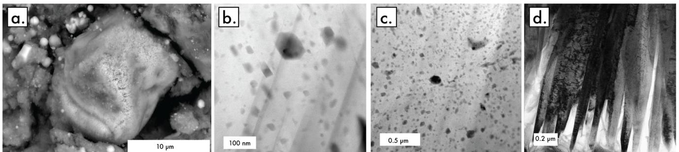
Figure 1. Backscattered electron (a), dark-field STEM (HAADF, b-c), and bright-field TEM images of the spherulitic magnetite analyzed in this study. The TEM data show the texture of the radiating fibers and the random distribution of euhedral to subhedral pores.
