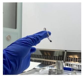
**Figure 1.** Glass vial containing Lunar regolith collected during the Luna 24 mission.
