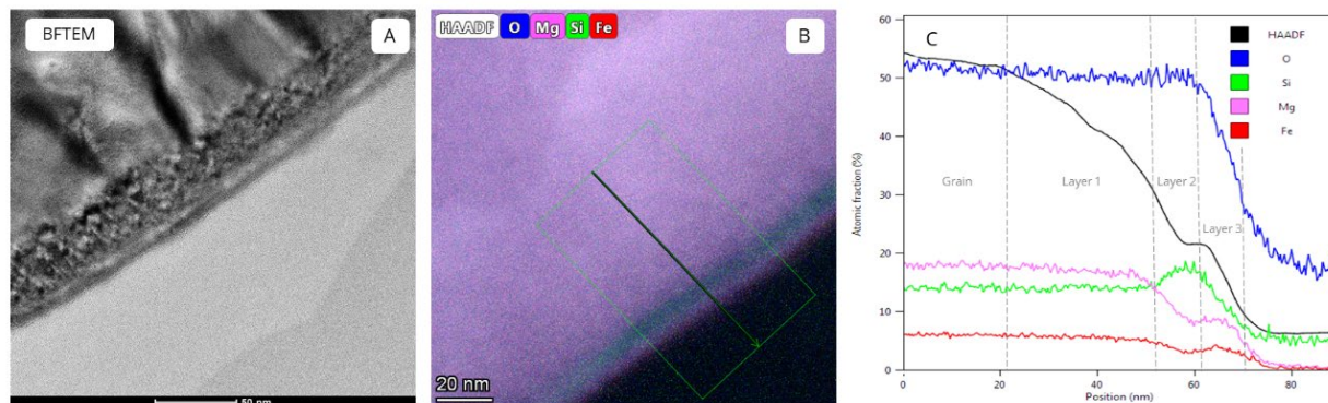
Figure 1. Space weathered rim on olivine grain. a) Bright field (BF) TEM image shown the ~50 nm mottled rim on olivine. b) High-angle annular dark field image overlain with EDS maps (O, Mg, Si, Fe). c) EDS line scan showing the chemical layering of the rim.
