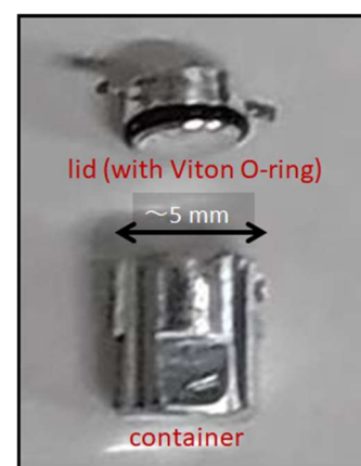
Figure 3. The small weighing container developed for the Hayabusa2 initial analysis.
