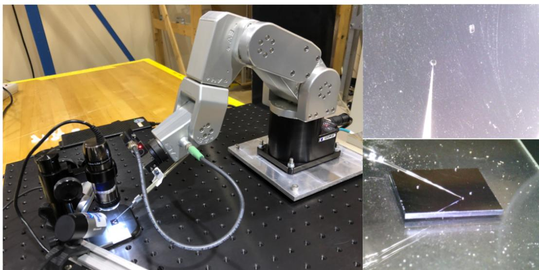
Figure 1: Meca500 robot arm manipulating 0.2mm magnetite particles on  $1\text{cm}^2$  silicon chip.
