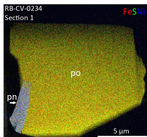
Fig. 1. Composite TEM X-ray element map (RGB=FeSNi) of RB-CV-0234 FIB Section 1; where po = pyrrhotite and pn = pentlandite.
