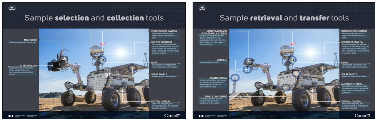
Figure 2: Sample collection and retrieval configurations of CSA's Mars Exploration Science Rover (MESR) prototype (Image Credit: CSA)
