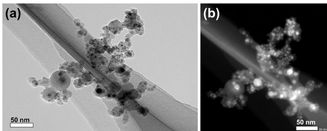
Figure 1. (a) TEM image and (b) STEM-HAADF image of metal embedded amorphous silicate grains produced in tangential plasma flame condition at 70 kPa.
