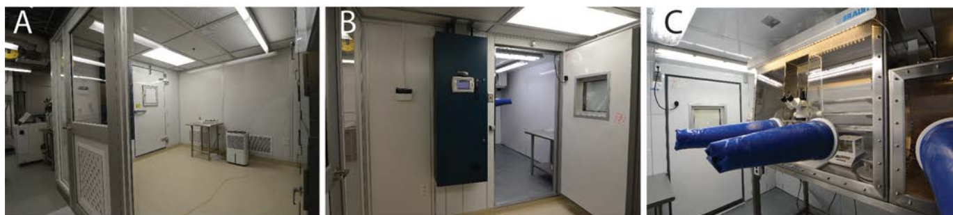
Figure 1. The Subzero Curation Facility at the University of Alberta, consisting of a Class 1000 room temperature anteroom (A), and a walk-in freezer (B) in which an Ar glove box is housed (C).
